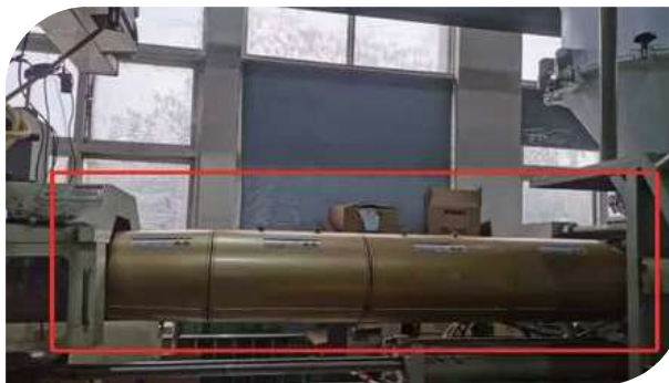
Install energy-saving heating coils on the injection molding machine to conserve electricity.
